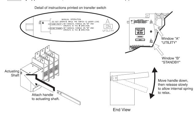
NOTE: Return handle to storage position in enclosure when finished with manual transfer
